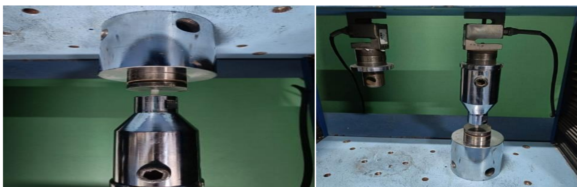
Fig. 8: Compressive strength test with Universal testing machine
