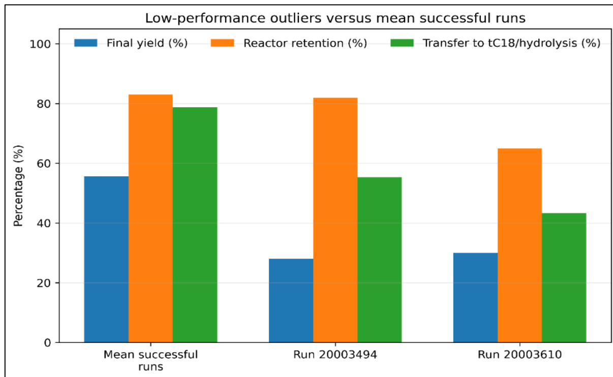
Fig 5 Comparison of Representative Low-Performance Production Runs Showing Efficient QMA Trapping But Reduced Downstream Radioactive-Material Transfer.
