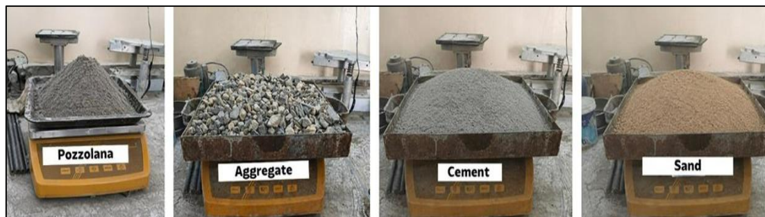
Fig 2 Materials Used to Produce Concrete
