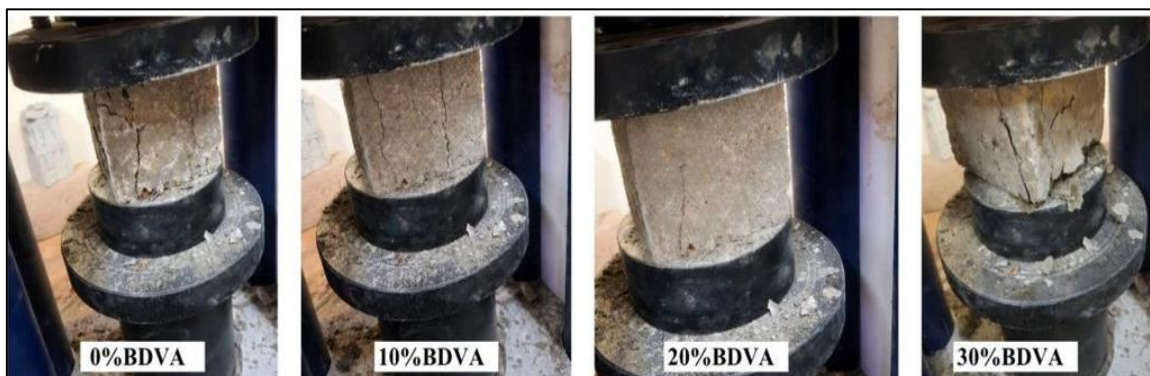
Fig 7 Failure Modes of Cube Specimens
