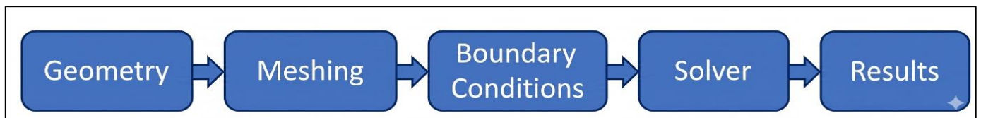
Fig 2 General Architecture of the Finite Element Analysis Procedure Implemented in Autodesk Simulation Mechanical 2015.
