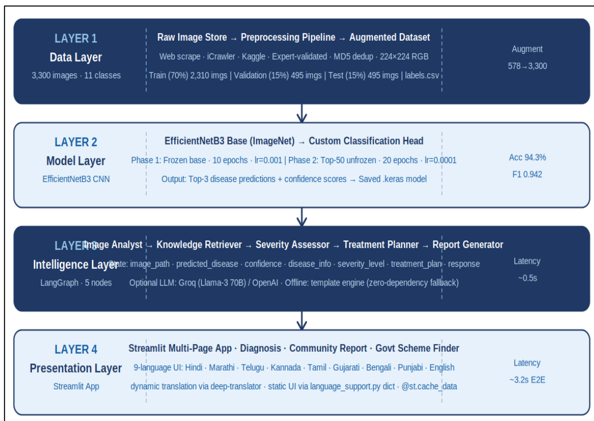
Fig 2 LAHMS Four-Layer System Architecture — Data, Model, Intelligence, and Presentation Layers with Component Detail
