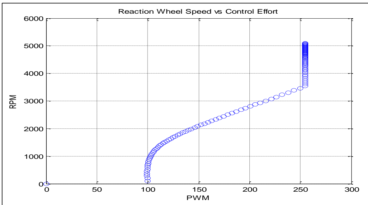
Fig 6 Reaction Wheel Speed vs Control Effort
