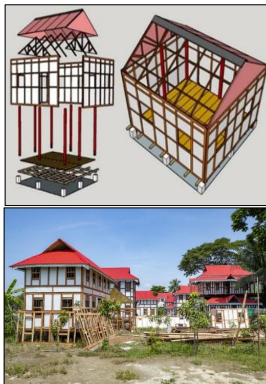
Fig 1 The Exploded 3D Model of Existing Building by Components; The Axonometric View of Existing Model (Source: Authors).
