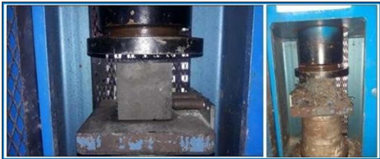
Fig 9 Compressive Test Cube Setup and Failure
