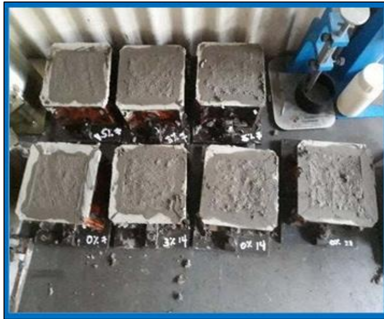
Fig 8 Preparation of Concrete Cubes
