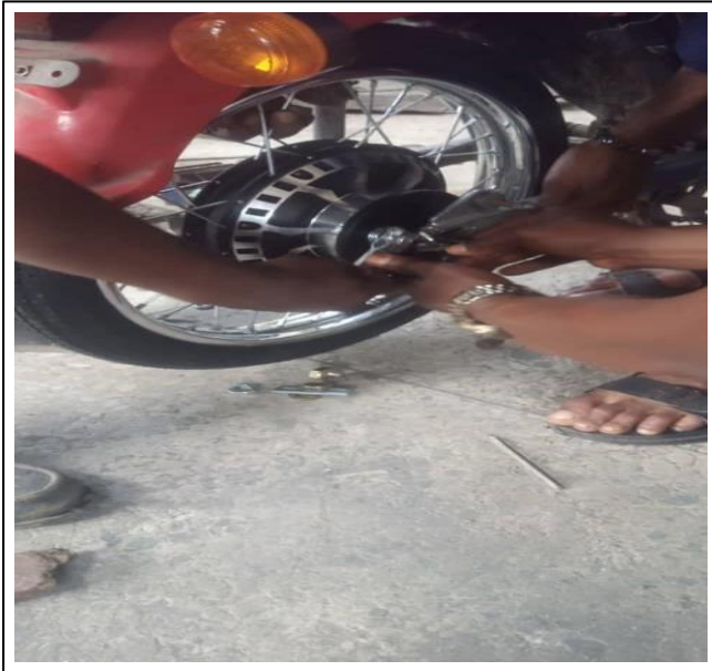
Fig 3 Picture of the Electric Motorcycle Brake being Fixed
