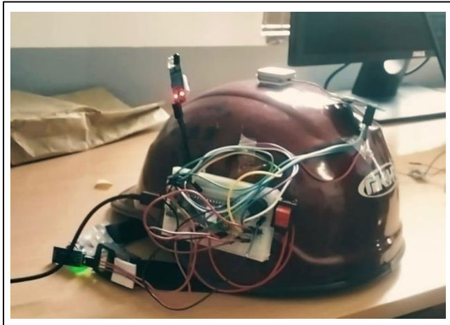
Fig 1 Safety Helmet Prototype with Integrated Sensors.
