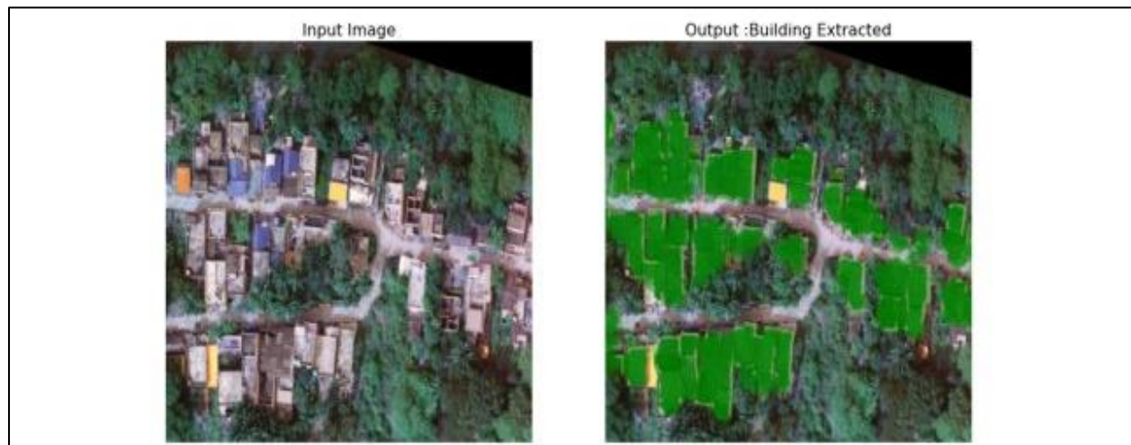
Fig 2. Input and Output of Building Extraction (Green Overlay) Results Over a Dense Mixed-Use Area
