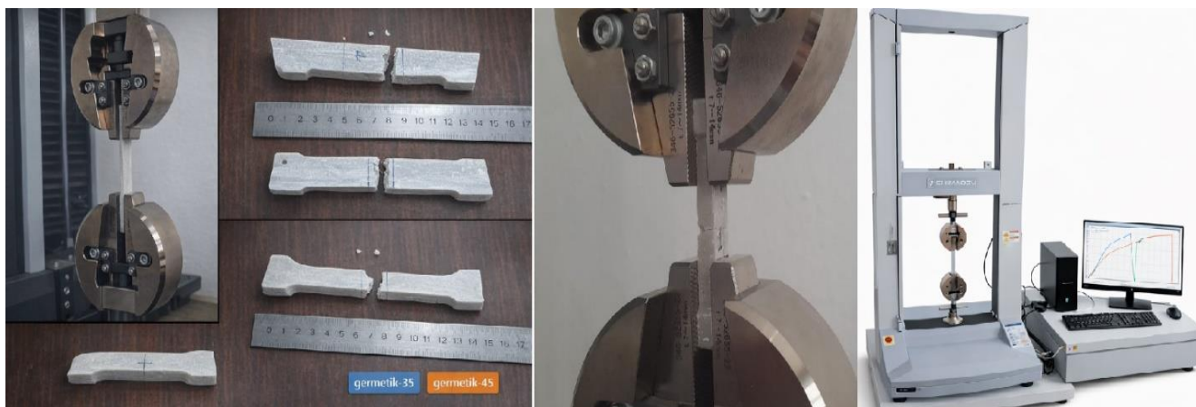
Fig 1. Chronological Tensile Testing Sequence and Post-Failure Profiles of Flame-Retardant-Modified Germetik-35 and Germetik-45 PVC Composites.
