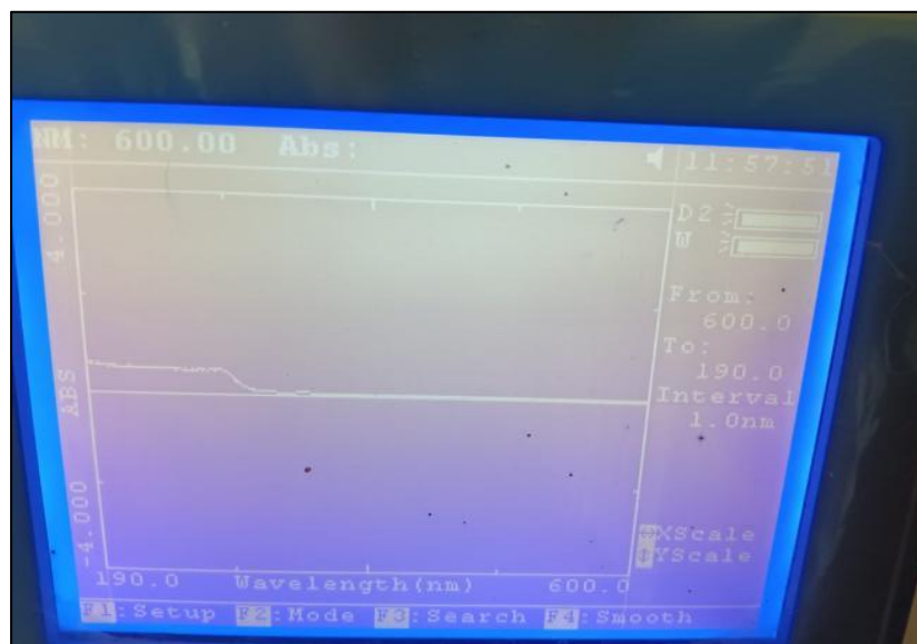
Fig 3B UV-Visible Spectra of Phenolphthalein, Basic Range (pH 8-12).
