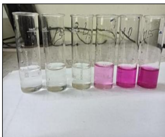
Fig 4A Colour Profile of Phenolphthalein Across pH 1.3-11.5.
