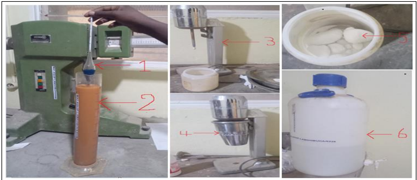
Fig 4 1. Hydrometer 2. Test Tubes 3. Mechanical Stirrer 4. Container 5. Deflocculant 6. Demineralized Water (Distilled Water)
