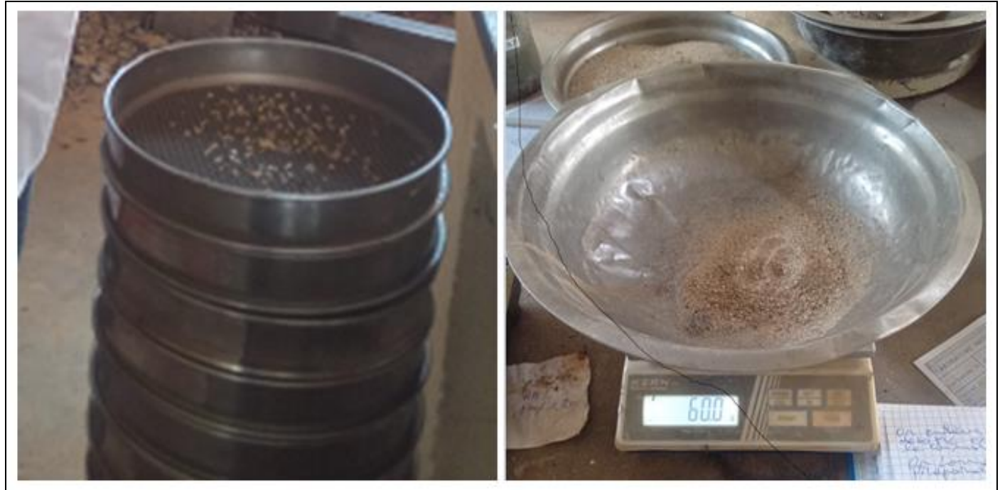
Fig 3 Series of Sieves and Scales Accurate to \pm 0.1\% .
