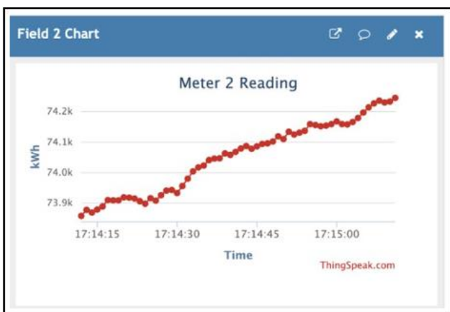
Fig 9 Readings of both meters in a specific time interval from Thing Speak Cloud
