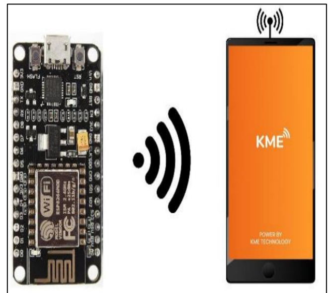
Fig 5 Wi-Fi Connection between ESP8266 and Kmesmart App
