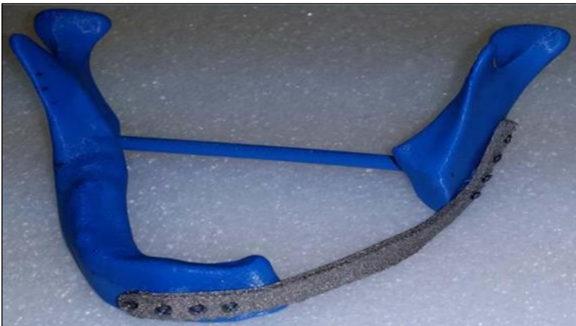
Fig 5 - Customized Titanium Implant Fabricated using EBM
