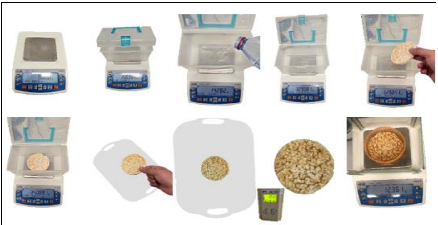
Fig 6 ASTM D570 Test Overview
