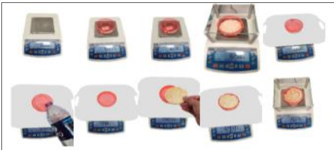
Fig 7 Archimedes Density Test Procedure
