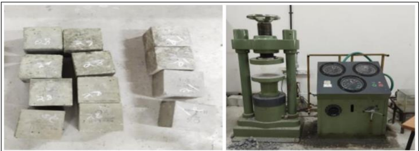
Fig 3 Concrete Cubes and Compression Testing Machine
