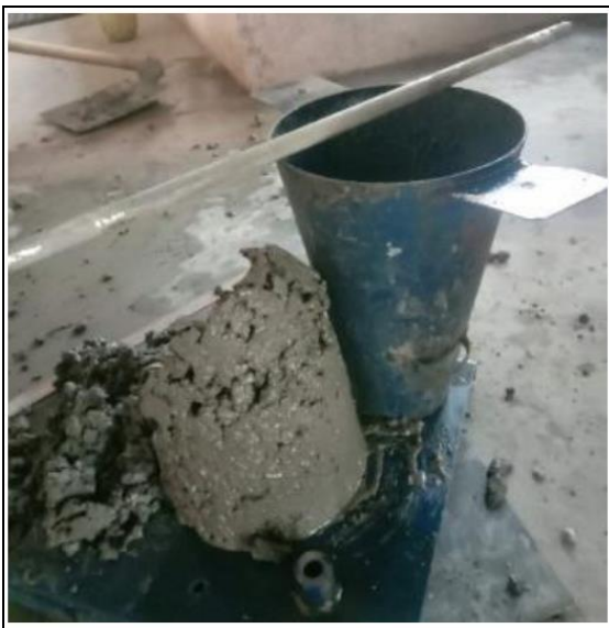
Fig 2 Slump Cone Test
