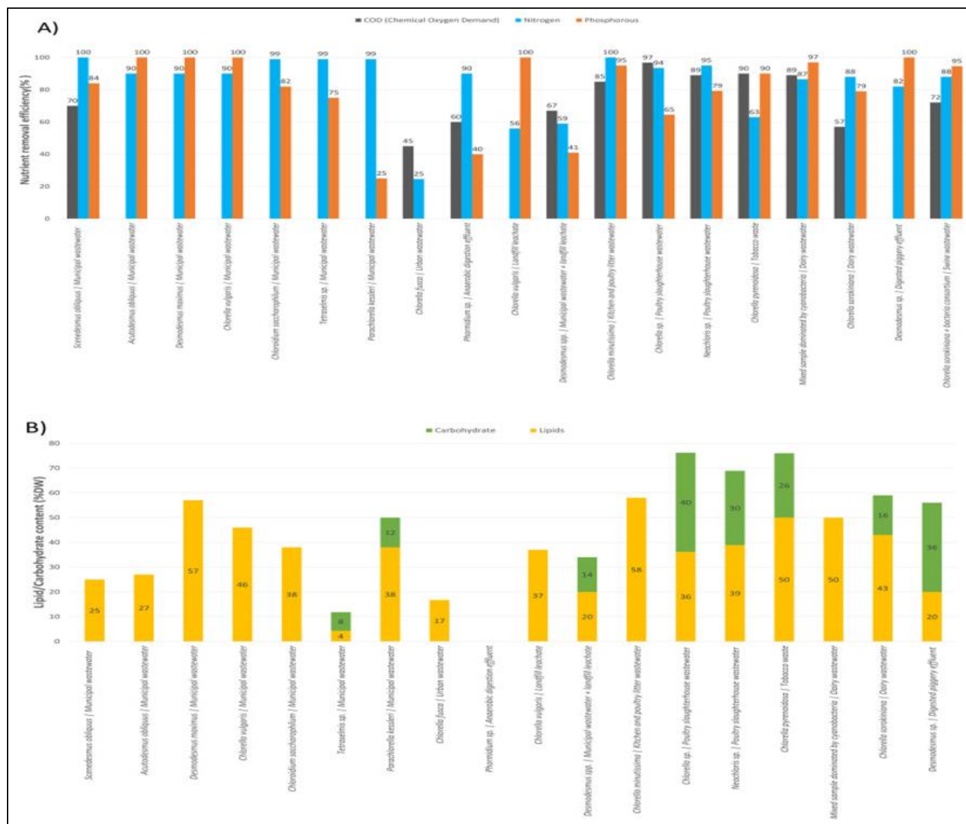
Fig 15 A) The nutrient removal efficiencies of microalgae grown in various waste streams, as well as their lipid and carbohydrate compositions, are presented here. Data for the figures are derived from studies on Nannochloropsis gaditana cultivated in municipal wastewaters, which produced 93.4 mg/g of bioethanol when fermented with yeast. In another study, Batista et al. (2015) grew Scenedesmus obliquus *, Chlorella vulgaris *, and a naturally occurring algal consortium C (comprising Chlorella *, Scenedesmus *, Chaetophora *, and Navicula *) in urban wastewater. As the nutrients in the culture media were removed due to nutrient recovery, the microalgae were left in the wastewater for an additional two weeks. This allowed them to synthesize high levels of sugars under nutrient-depleted stress conditions. The resulting sugar content was measured as 42%, 21%, and 28% ash-free dry weight for S. obliquus *, C. vulgaris *, and Consortium C, respectively. When fermented with Enterobacter aerogenes *, the volumes of biohydrogen produced were 56.8, 40.8, and 46.8 mlbio-H 2 /g volatile solids for S. obliquus *, C. vulgaris *, and Consortium C, respectively. S. obliquus * showed 98% ammonium, 100% phosphate, and 54% COD removal from urban wastewater, while C. vulgaris * achieved 96% ammonium and 7% phosphate removal but saw an increase in COD by approximately 37%. Consortium C, on the other hand, demonstrated nearly 100% removal of both ammonium and phosphate but did not significantly reduce COD.
