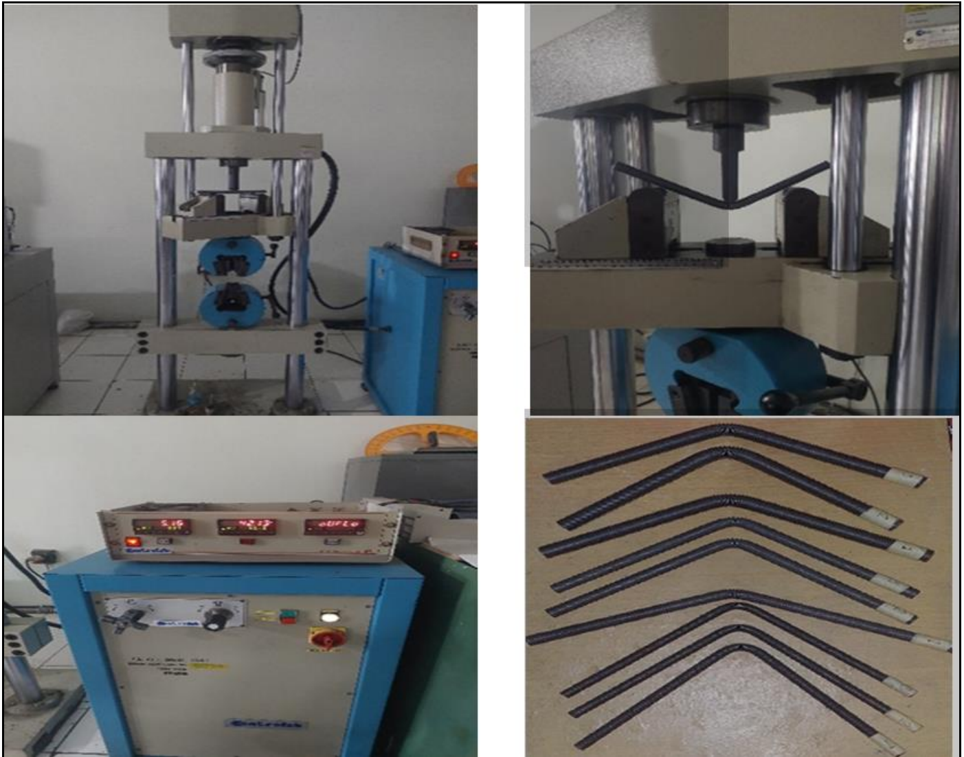
Fig 12 Bolt Flexural Yield Strength Testing
