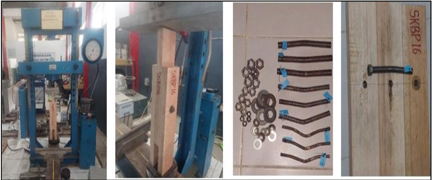
Fig 13 Testing the Joint of Two Wood Sections
