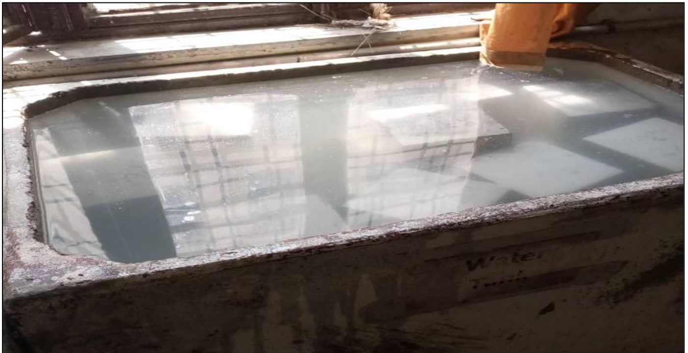
Fig 8 Curing in a Water Tank
