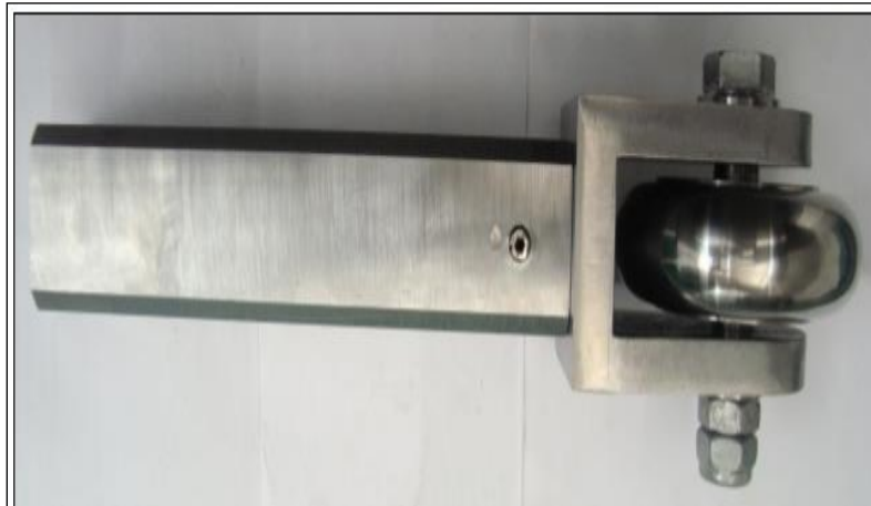
Fig 3 Actual Image to Existing Roller Burnishing Tool Actual Image to Existing Roller Burnishing Tool.
