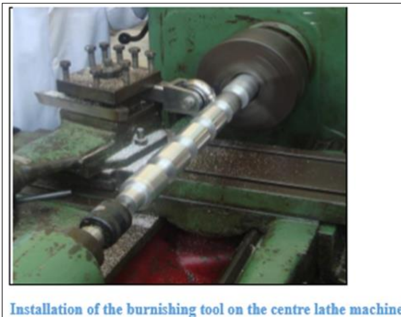
Fig 4 Actual Image to Existing Roller Burnishing Process.
