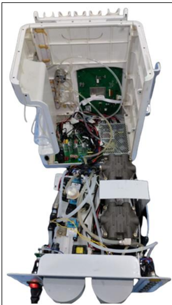
Fig 4 Internal Components of the Hydrafacial Machine Including Pump, Solenoid Valves, and Piping Network.
