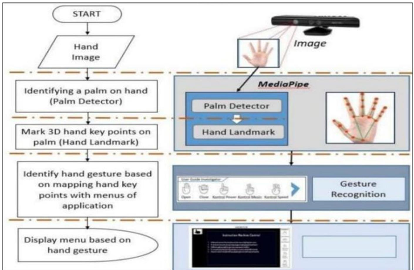
Fig 2 System Architecture
