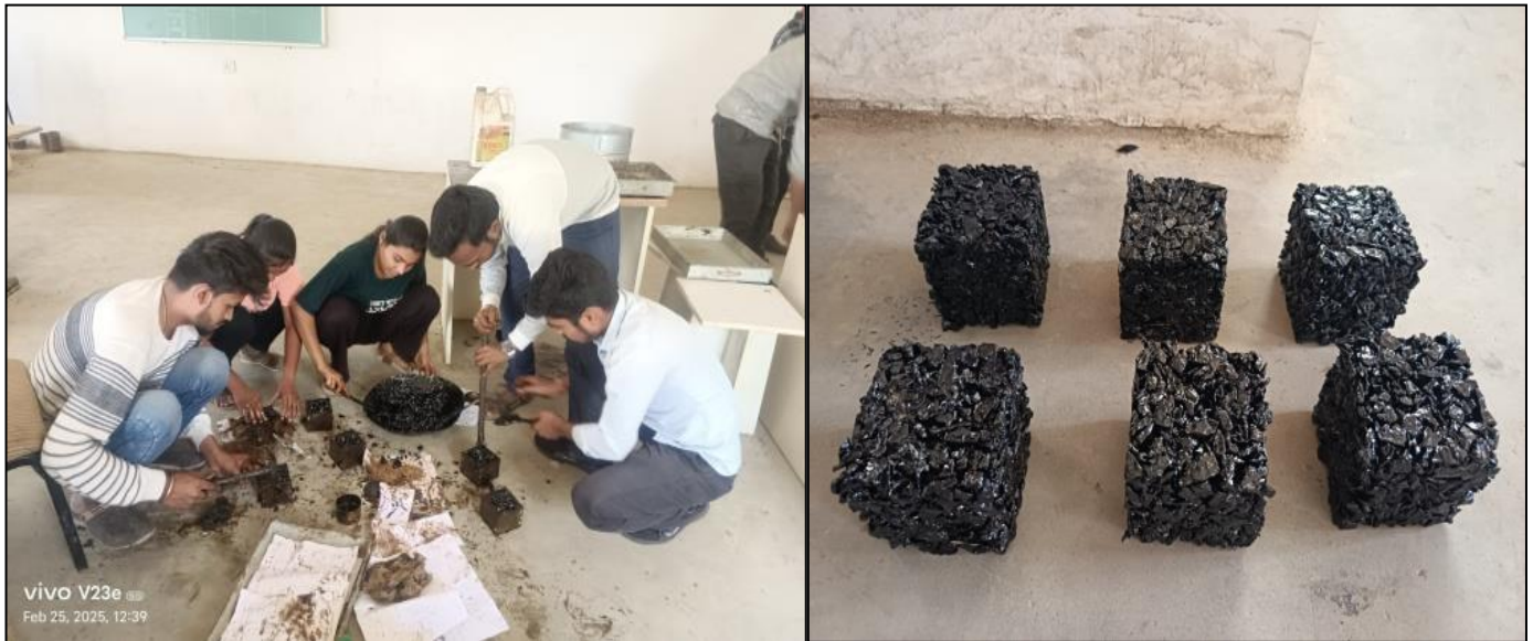
Fig 9: Cube Casting on Plastic-Bitumen-Aggregate Mixture
