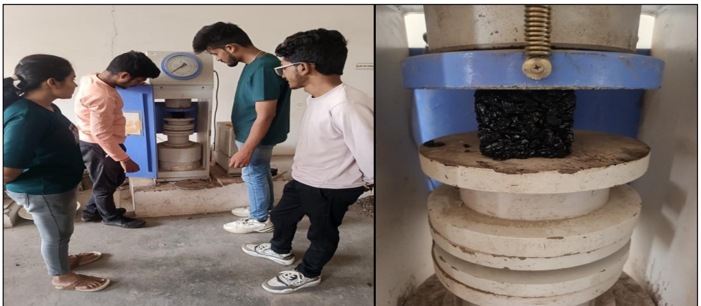
Fig 10: Compressive Strength Check on Cube of Plastic-Bitumen-Aggregate Mixture
