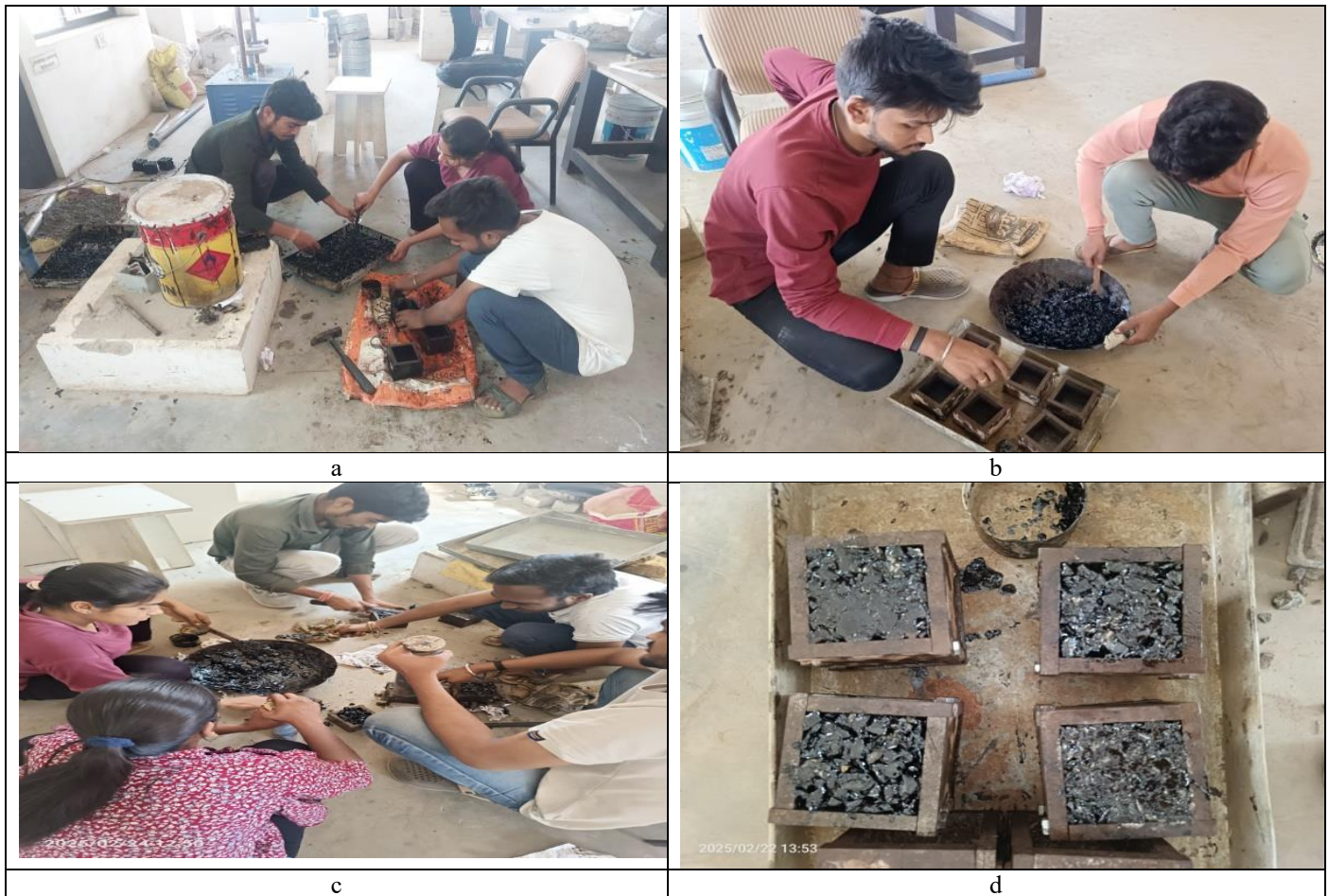
Fig 8: Cube Casting on Bitumen-Aggregate Mixture
