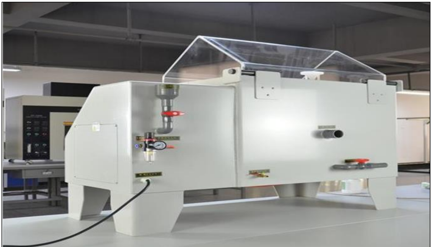
Fig 2 ASTM B 117 Salt Spray Chamber
