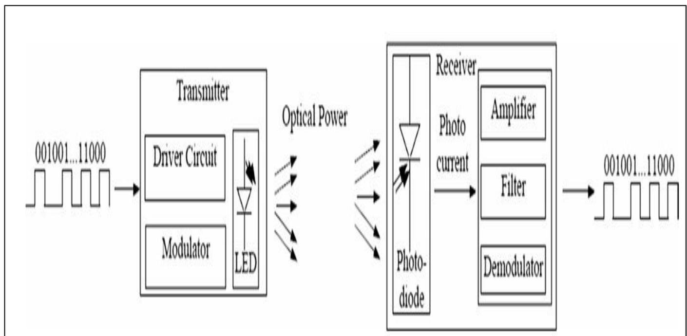
(a) Block diagram of the VLC communication process
