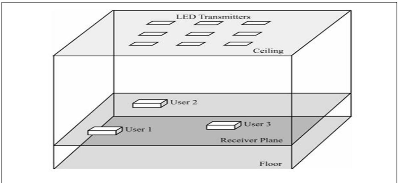
(b) Spatial arrangement of LED transmitters and user receivers within an indoor environment
