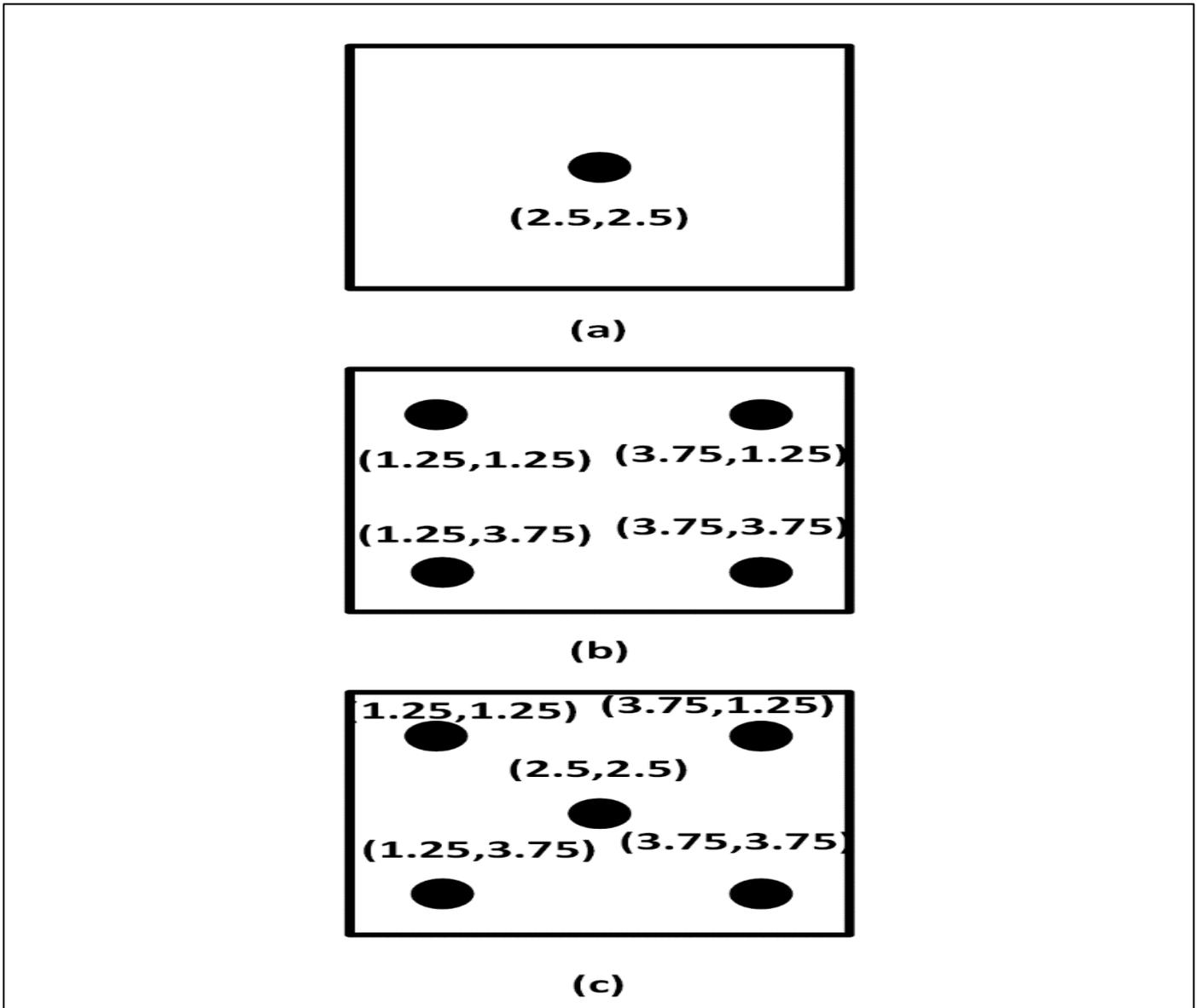
Fig 3 The Position of Leds When (A) Single Transmitter (B) Four Transmitter (C)Five Transmitter
