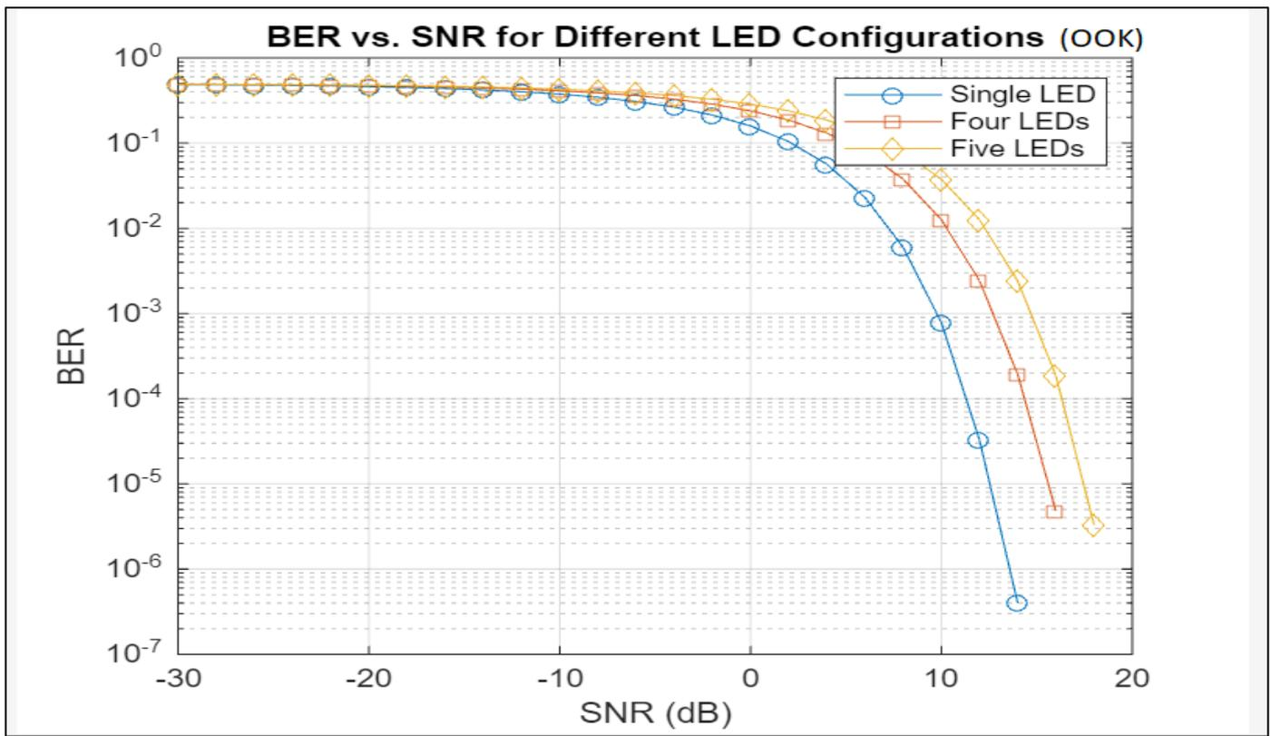
Fig 12 BER versus SNR Curve for OOK
