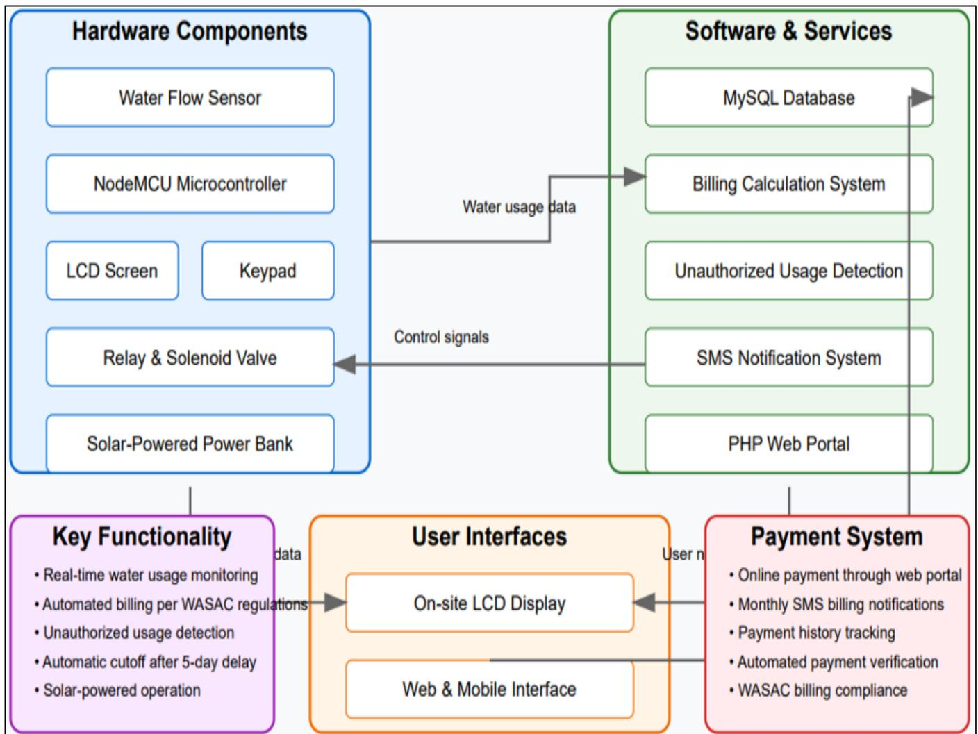
Fig 5 System Architecture
