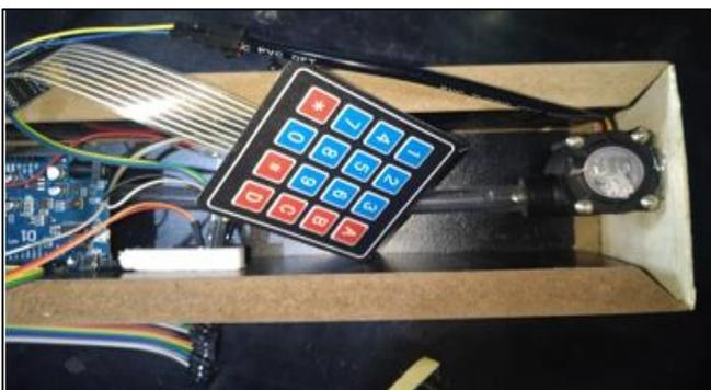
Fig 16 Keypad as Fetching Input Level
