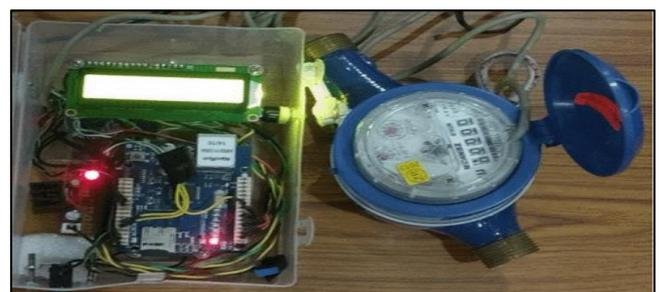
Fig 2 Smart-Meter Prototype with External
