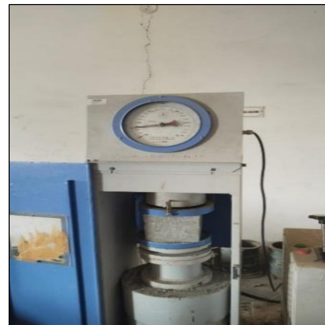
Fig 3: Testing Compressive Strength of Cubes
