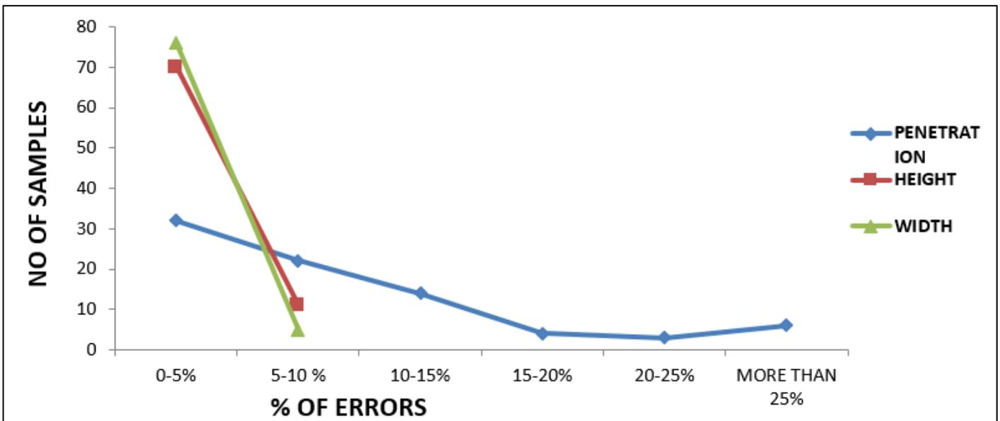
Fig 6 Accuracy Analysis of Bead Penetration, Height and Width
