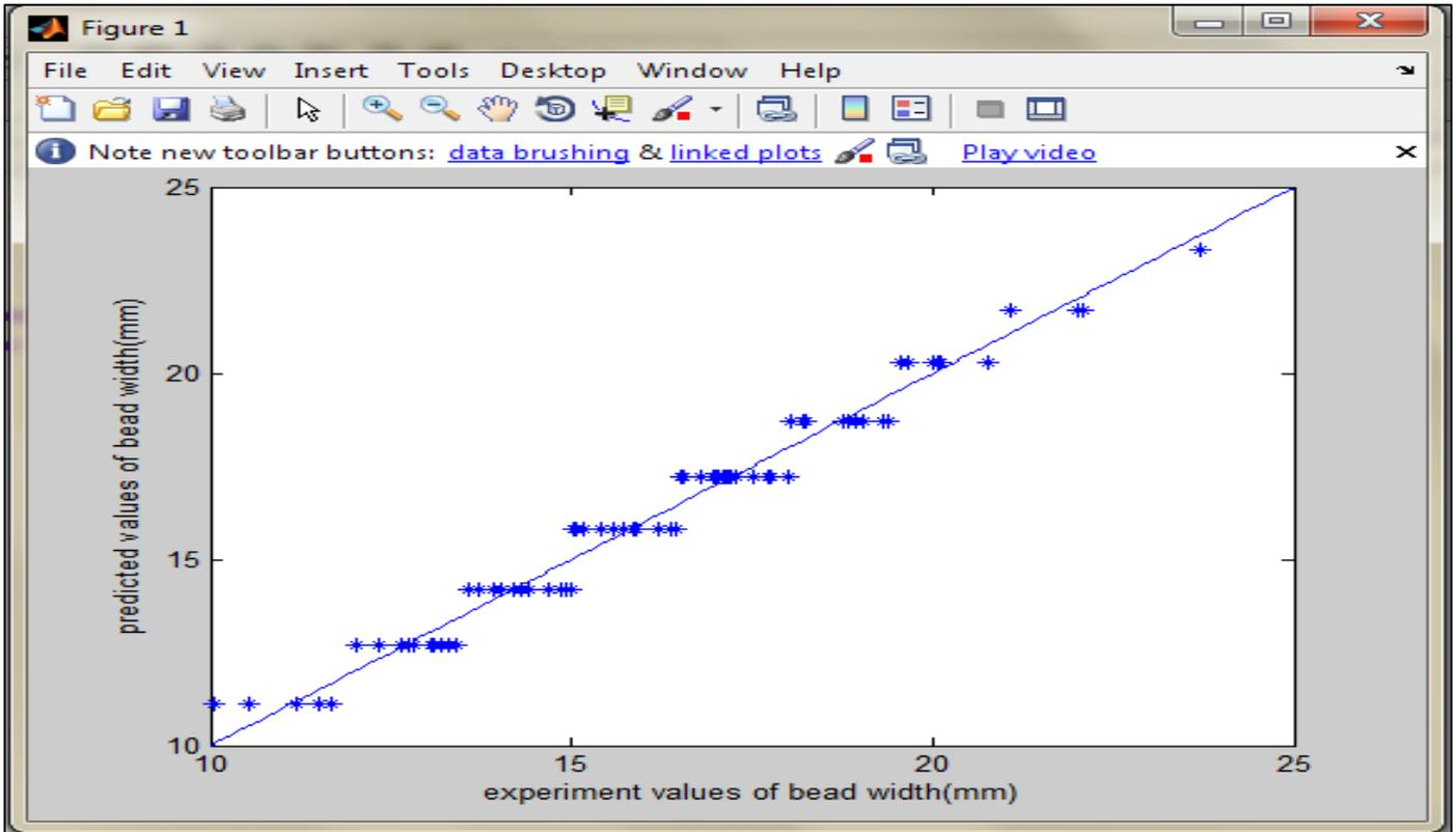
Fig 5 Scatter Diagram of Bead Width (W)
