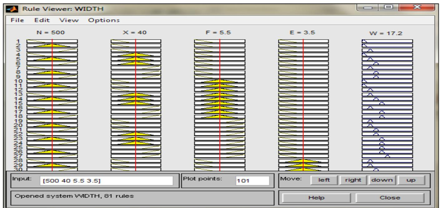
Fig 2 Rule Viewer of Bead Width (W)
