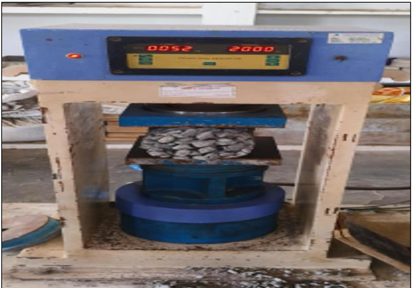
Fig 6 Tensile Strength Test of Pervious Concrete
