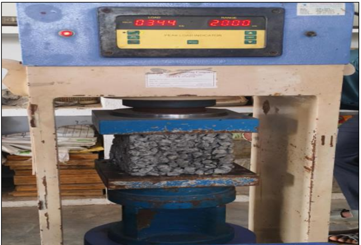
Fig 4 Compressive Strength Test of PC
