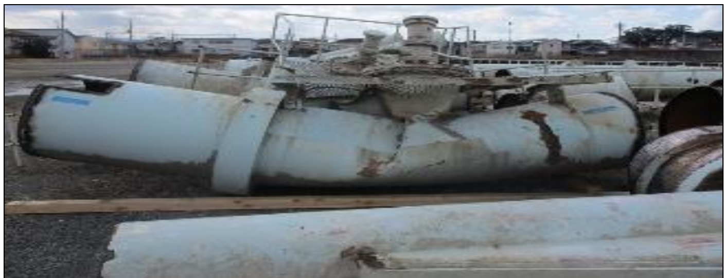
Fig 5 Damaged Air Valve Located in the Middle of the Span
