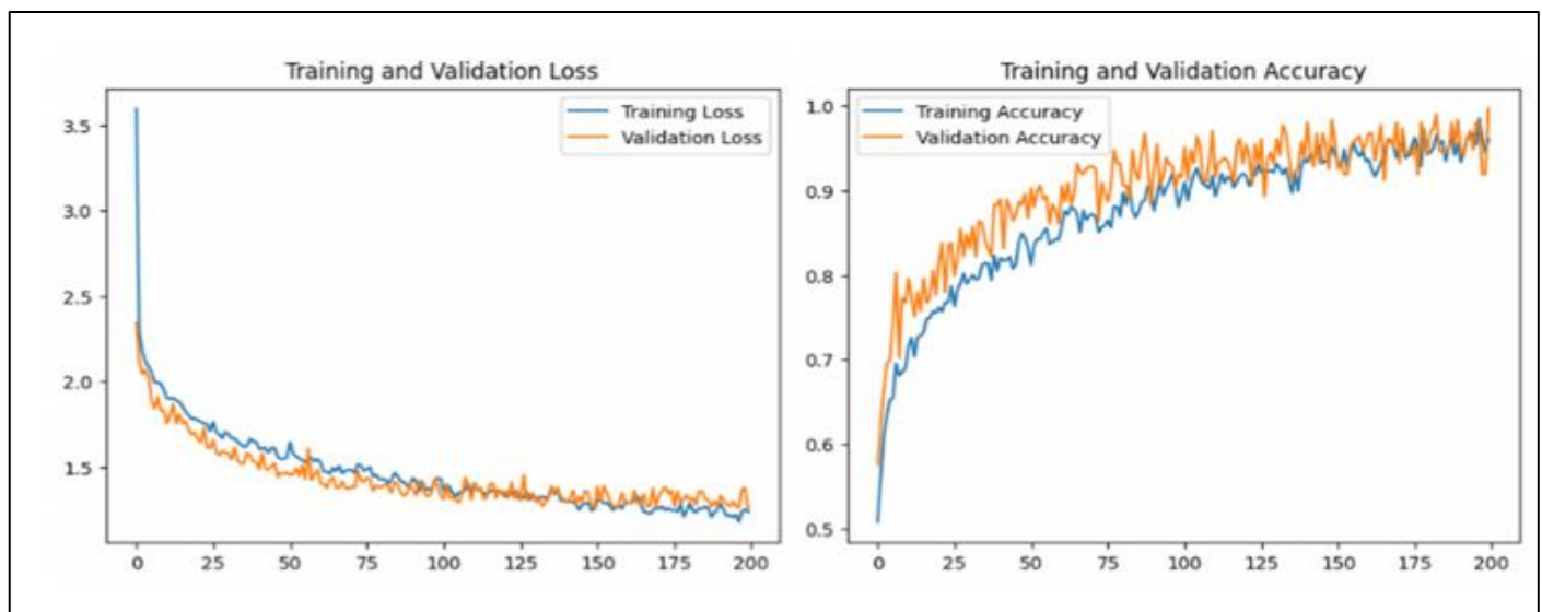
Fig 20: The Learning Curves Depicting Loss and Accuracy During the Training of the MobileNetV3 Model on Image Size 224x224
