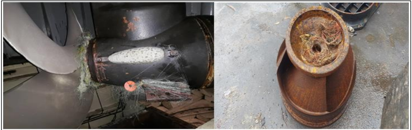
Fig 2: Left is the Impeller with Damaged Seal, Right is Propeller Caught Fishing Lines
