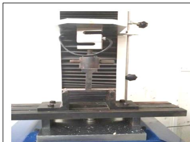
Fig 6: Flexure Test on UTM
