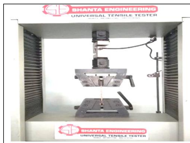
Fig 5: Tensile Test on Universal Testing Machine
