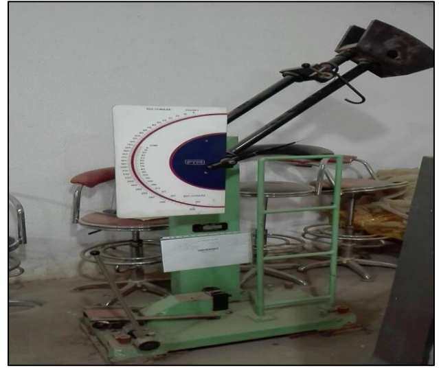
Fig 3 Shows the Installation of the Charpy Shock Test Device.
