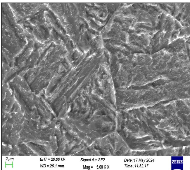
Fig 11: Microstructure of the Weld Region
