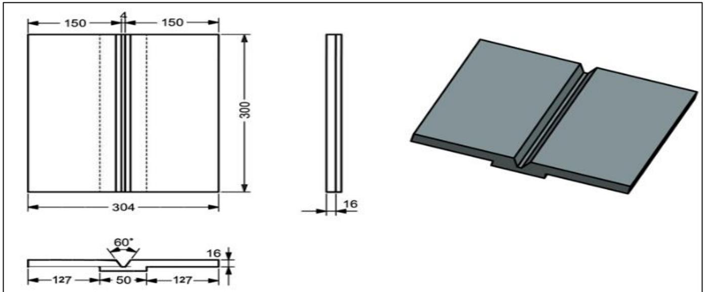
Fig 1: Base Metal Plate for FCAW Welding with Groove
