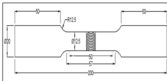
Fig 4: Tensile Specimen Preparation as Per ASTM E8 Standards
