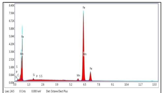
Fig 13: Typical EDAX Spectrum of the Inclusions
