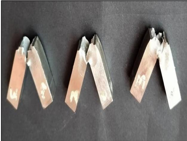
Fig 7: Notch Specimen after the Impact Test
