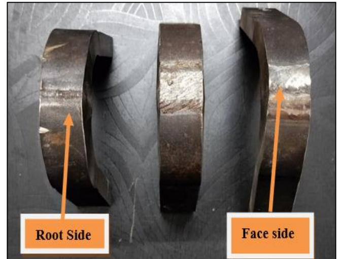
Fig 8: Welded Sample after Bending
