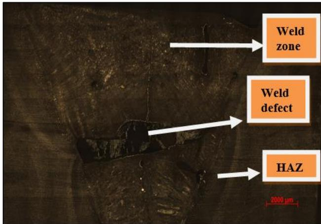
Fig 9: Optical Micrograph of FCAW Welded Joint
