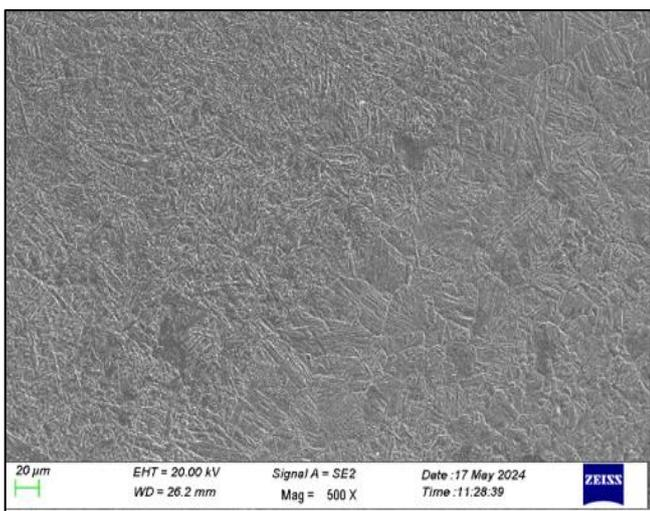
Fig 10: Microstructure of at the Interference of Base Metal and Weld Region
