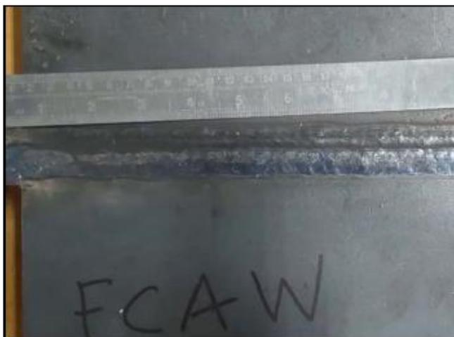
Fig 3: FCAW Welded Specimen
