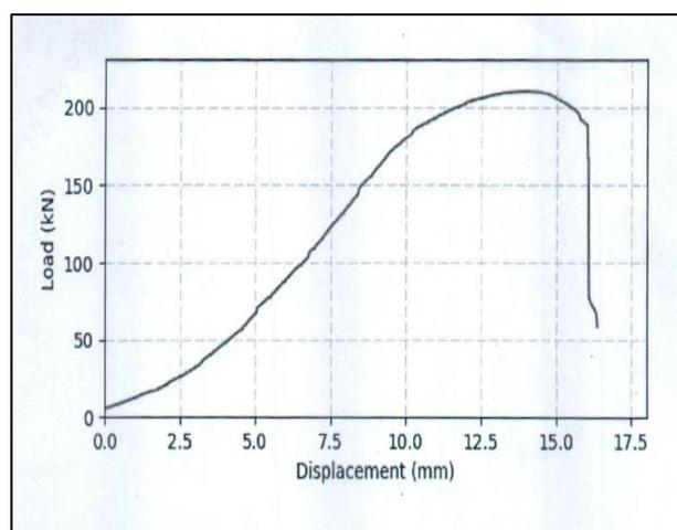
Fig 6: The Load to Displacement Curve for Welded Joints
