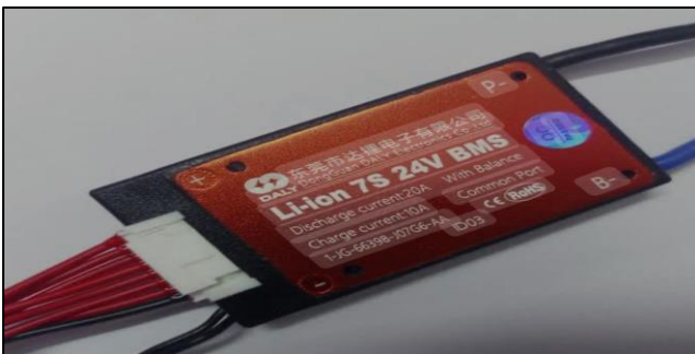
Fig 3: BMS (Battery Management System)
