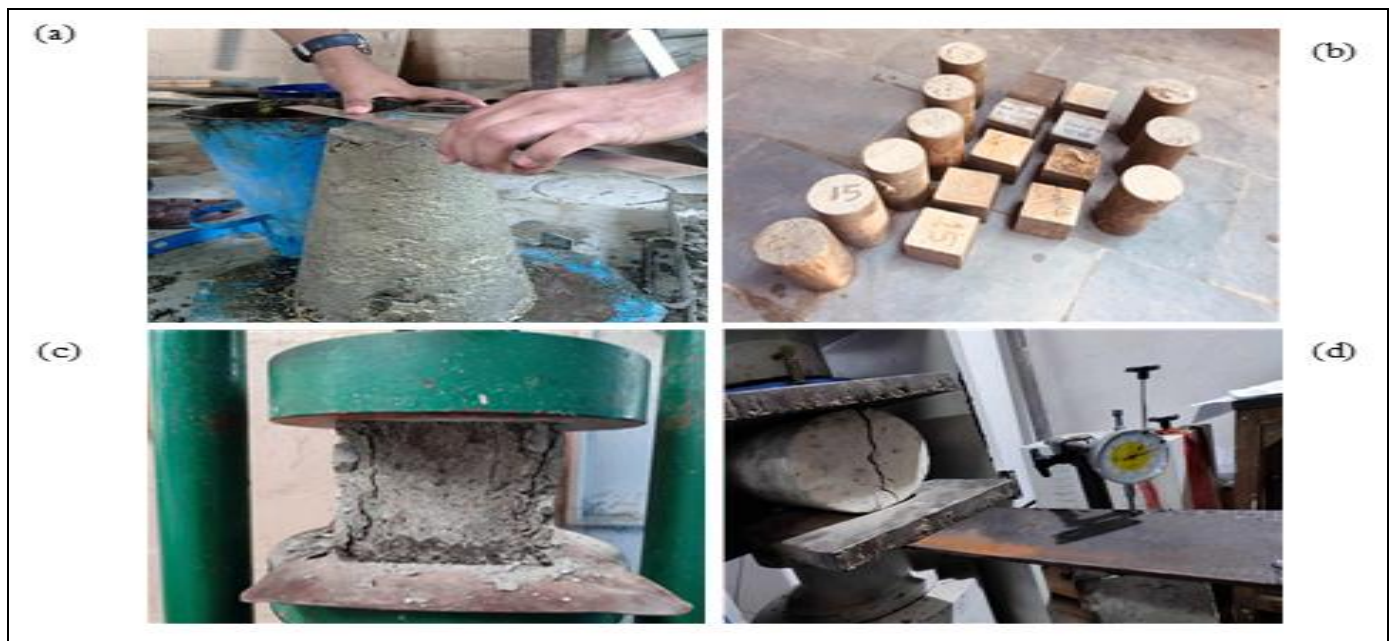
Fig 2: Fresh and Hardened Properties Test (a) Workability Test (b) Prepared Specimens (c) Compressive Strength Test (d) Splitting Tensile Strength Test
