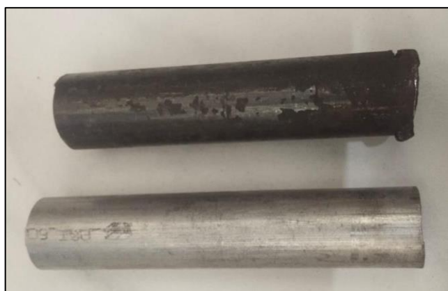
Fig 2: Aluminium and EN-8 Material before Turning Operation
