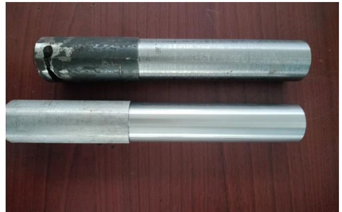
Fig 4: Aluminium and EN-8 Material After Turning Operation
