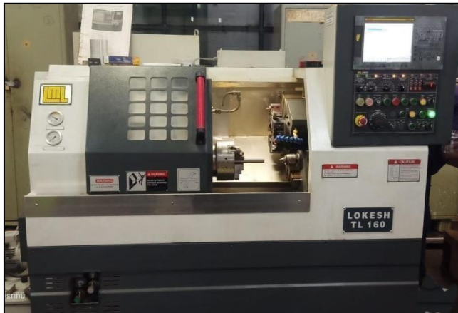
Fig 1: CNC Lathe for Turning Process
