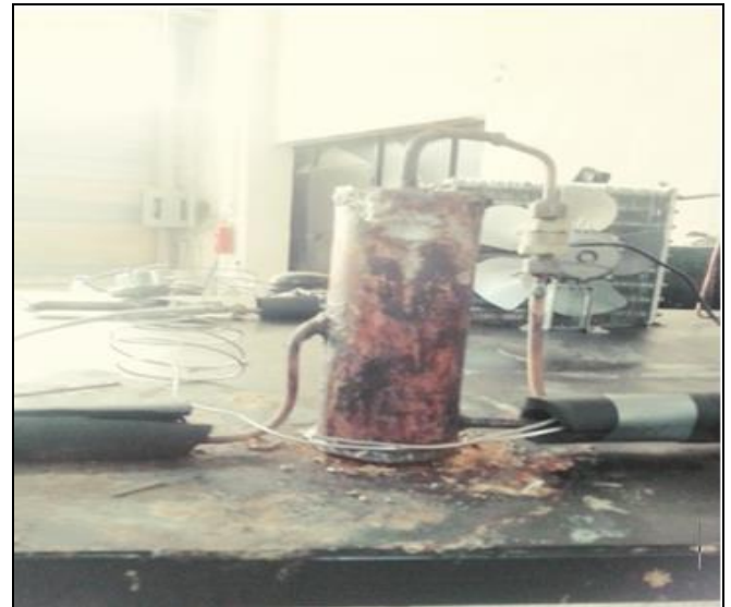
Fig 10: Shows the Tank to Collect the Liquid Refrigerant
