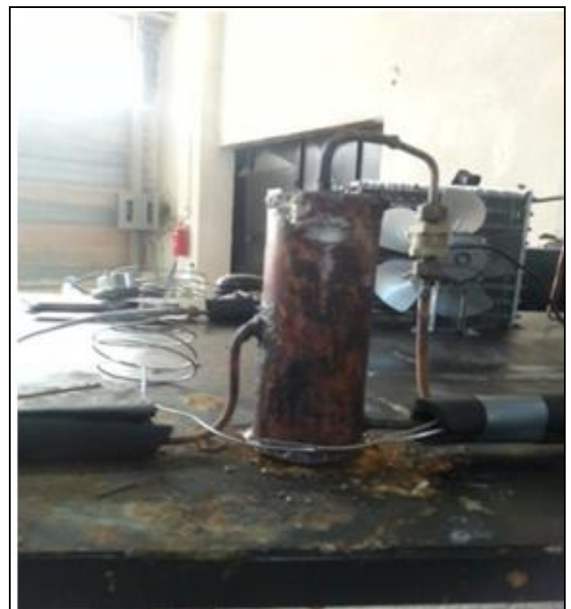
Fig 8: Shows the Liquid Collection Tank
