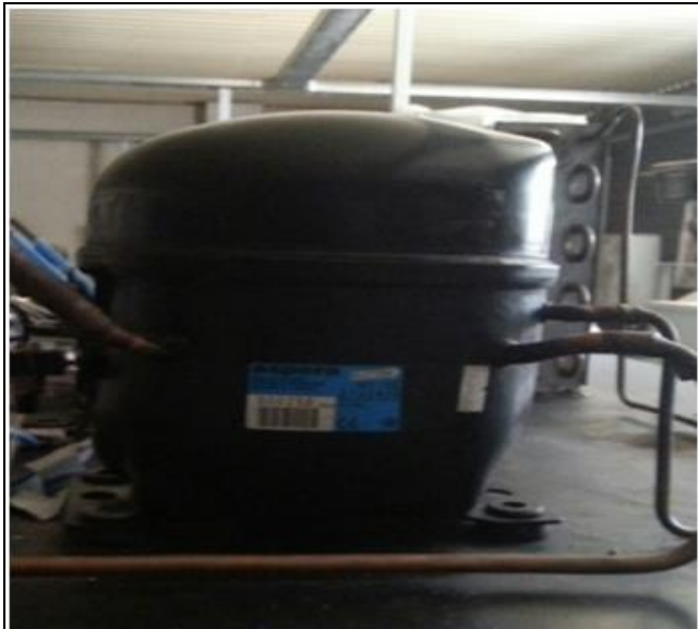
Fig 1: Shows the Compressor
