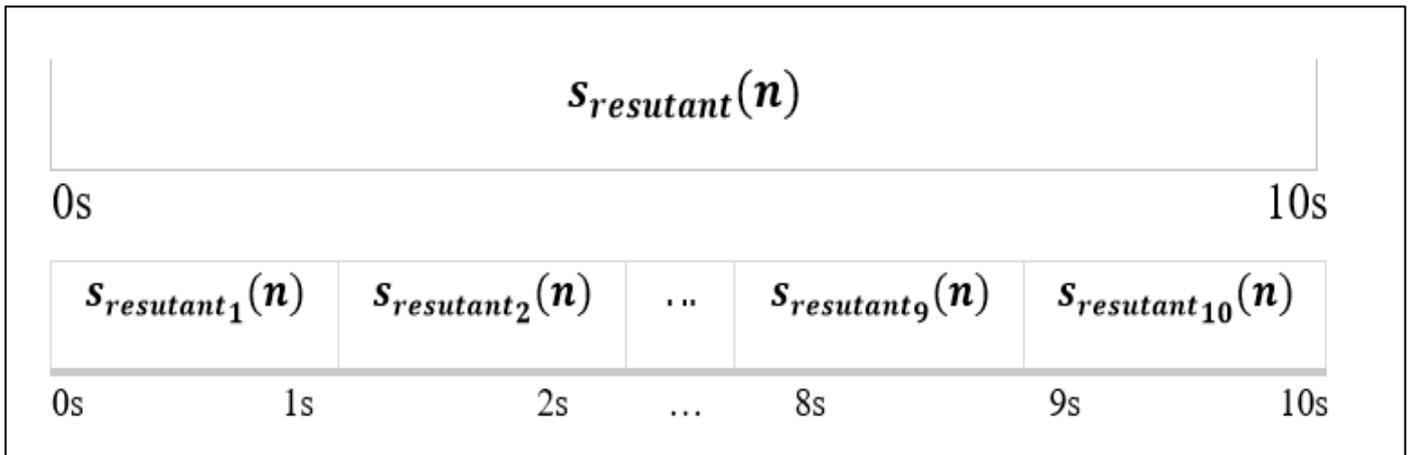
Fig 1 Segmentation of the Signal Resulting from Merging the Left and Right Channels
