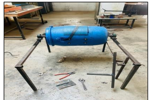
Fig 10 Final Model Foot Powered Laundry Machine
