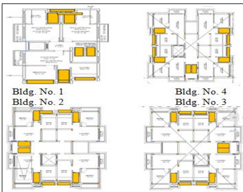
Fig 3 Typical Floor Plan for Bldg. 2,3,4 & 1 (Coloured Part Showing the use of Precast Slab)
