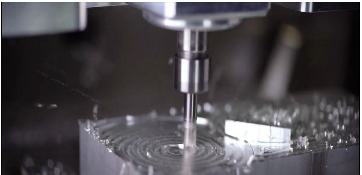
Fig 2: Aluminium Cutting Image of CNC Milling Machine
