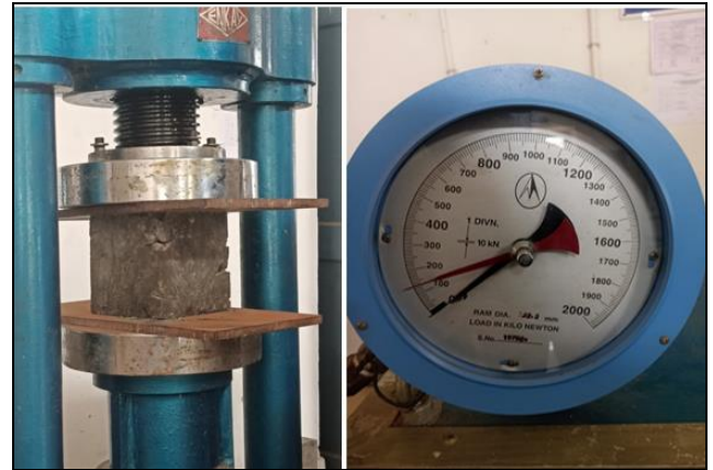
Fig 7: Compressive Strength Test Conducted
