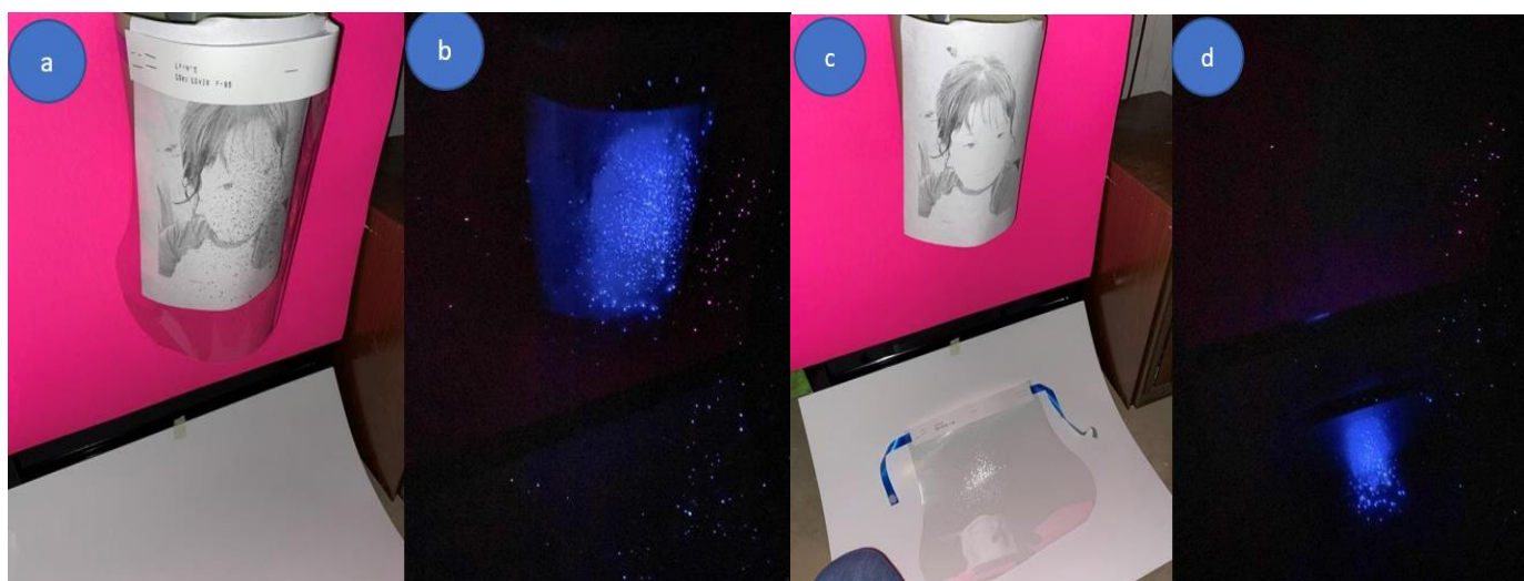
Fig 3: Macroscopic Droplet of Fluorescent Dye on “Pretend-Person” Exposed to Cough with Light on (a) and Light off (b) with Shield on and with Shield off. “Face Shield” Seemed to Have Completely Prevented Macroscopic Fluorescent Droplet from Reaching “Pretend Person’s” Face (c and d)
