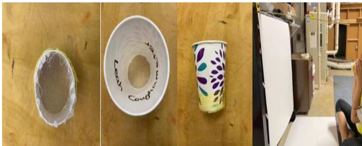
Fig 1(C): “Coughometer”. Junior researcher posed but never used “Coughometer”. The Bottom of the “Coughometer” was Soaked in Inkpad (Figure 1C) and Coughed Thought it to Simulate Propulsion of Macroscopic Oropharyngeal Droplets
