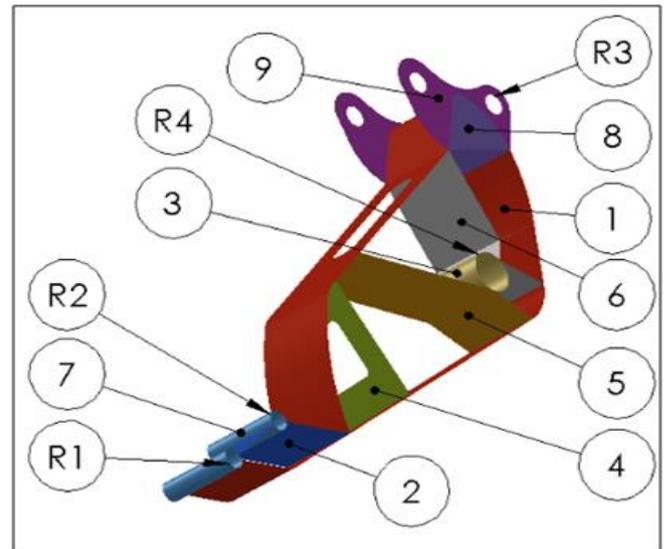
Fig 6 the New Model with Various Components
