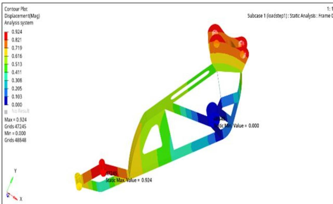
Fig 8 Max Displacement for the Arm is 0.9mm
