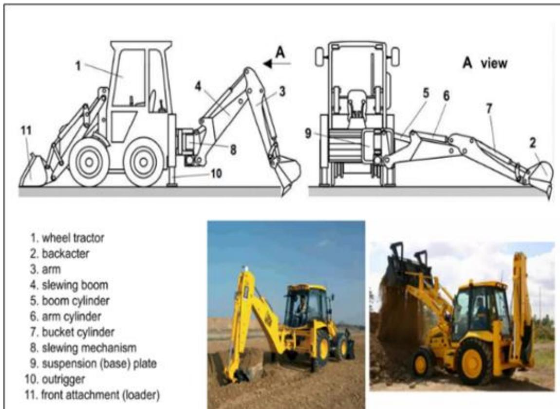
Fig 1 The Backhoe Excavator Components
