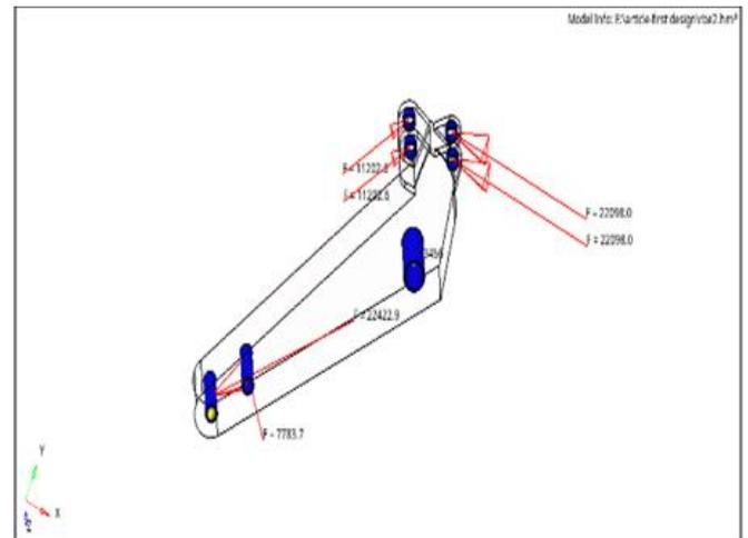
Fig 4 Applying the Boundary Conditions on the Arm
