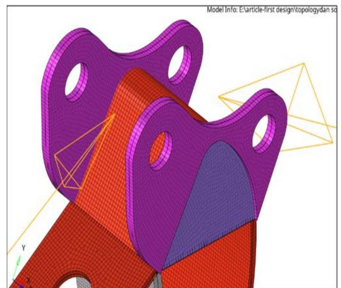
Fig 7 Meshing and Giving Initial Thickness for all Components
