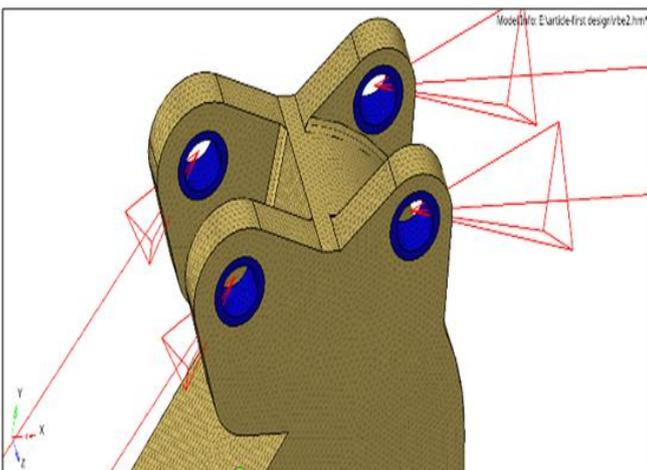
Fig 3 Meshing the Body of the Arm
