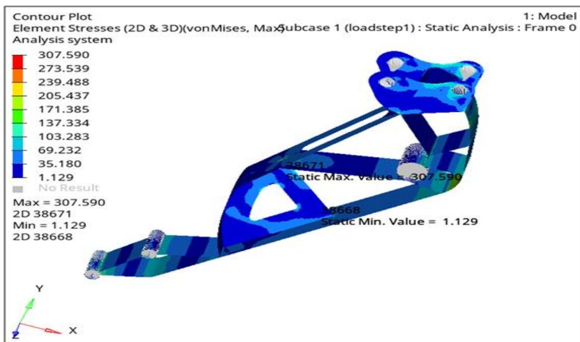
Fig. 9 Von Mises Stress for the Arm
