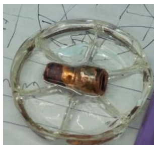
Fig 3. 0.61mm Thick Copper Pipe
